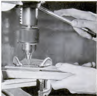
The slides are stacked and clamped between pieces of wood while the holes for the binding are drilled
